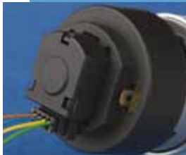
gear-motors with two-phase Hall-effect 90° encoder
