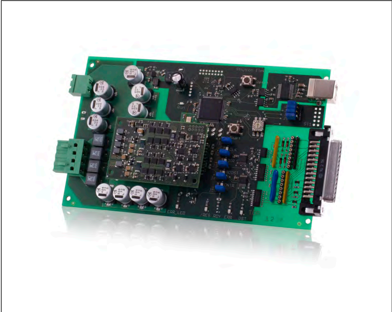
Fig. 1: EVA-APS carrier module with plugged APS module plugged in
